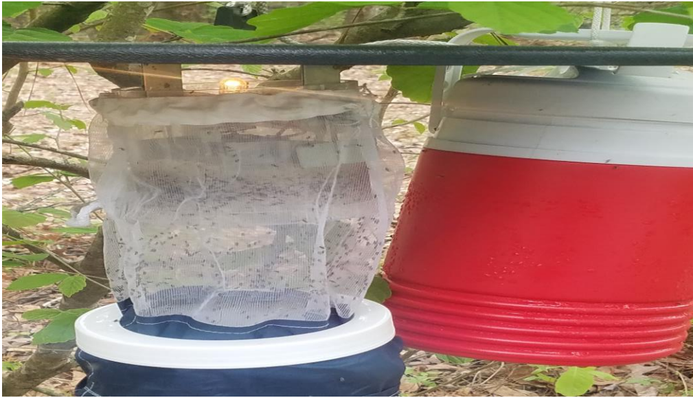
Figure 3.3 CDC CO 2 -baited light trap with black flies
